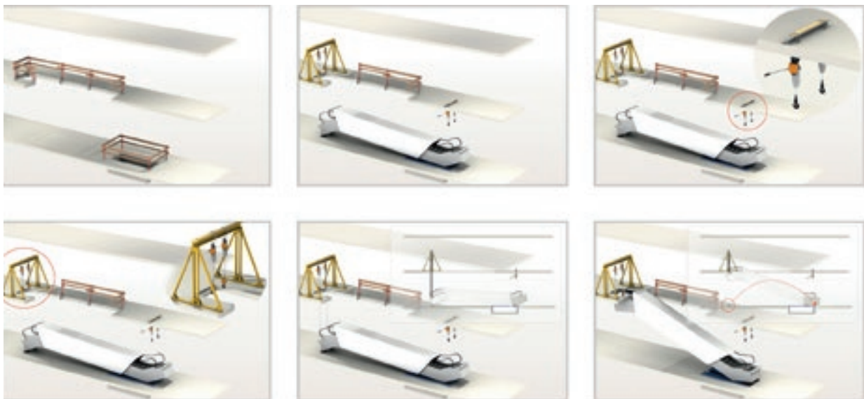
Figure 8.2 Installation in one section using A-frames
