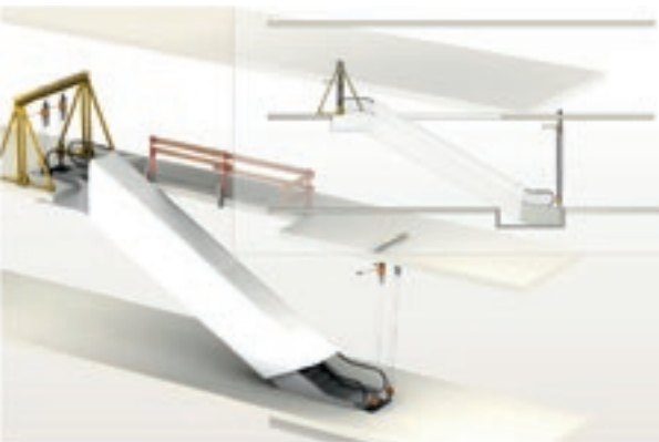
Figure 8.5 Installation using a lifting frame
